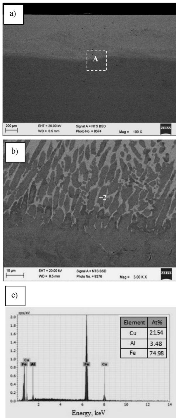
Fig. 6. Microstructure of the single layer clad of CuAl9Fe3 bronze on the substrate of S355J2 steel produced by laser cladding (a), transverse section unetched; b) detail “A” from the Fig. a - microstructure of CuAl9Fe3 bronze, under SEM examination; c) microanalysis obtained from point (2)
