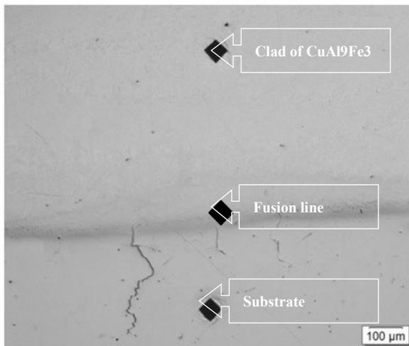
Fig. 7. Cross-section of the single layer clad of aluminum bronze CuAl9Fe3 on the steel substrate with marked points of hardness measurements
