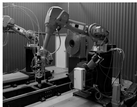
Fig. 2. A view of the robotic stand equipped with a high power diode laser HPDL LDF 4000-30 LaserLine
