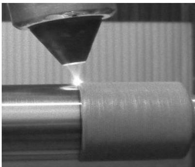
Fig. 3. A view of laser powder cladding process of the rod made of steel S355J2 by aluminum bronze using a high power diode laser HPDL
