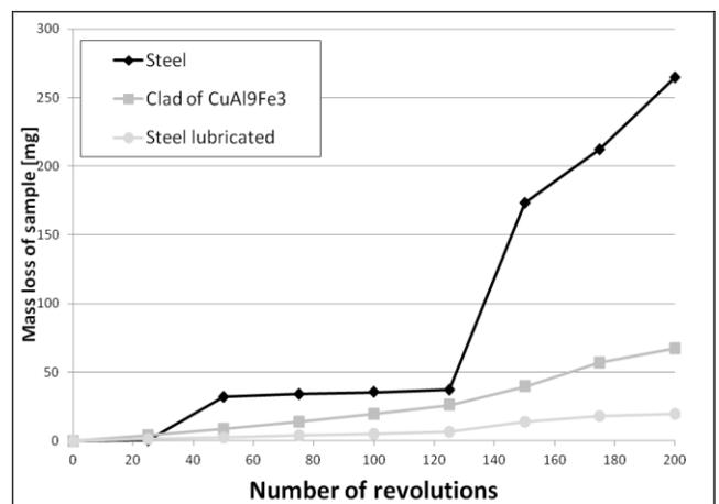
Fig. 9. The mass loss of tested samples after 200 revolutions, at the normal force 700 N
