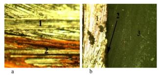
Fig. 12. Cortical EIs at X50 magnification: a - a cortical EI obtained by casting; 1 – metal base; 2 – copper layer; b – a cortical EI obtained by the rapid prototyping technology; 1 – copper layer; 2 – preliminary conductive layer; 3 – polymer base.
