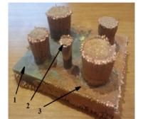
Fig. 8. Cortical EI: 1 – the primary conductive layer; 2 – copper build-ups; 3 – copper layer
