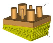
Fig. 3. Processing a CAD model of the EI for layer-by-layer building at the SLA - Envisiontec Perfactory XEDE installation: 1 - EI model, 2 - supporting devices
