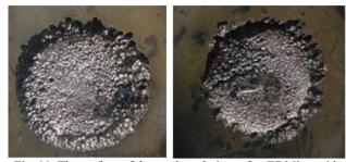
Fig. 11. The surface of the steel workpiece after EDMing with cortical EIs: a – imprint after treatment with cast EIs; b – imprint after treatment with EIs obtained through the RP technology
