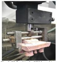
Fig. 9. EI fixed in the EDM machine. Processed material is grade 65C steel, GOST 14959 -79
