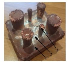
Fig. 7. A cortical EI obtained by casting after galvanic treatment: 1 – copper coating layer; 2 – uncovered areas; 3 – copper build-ups
