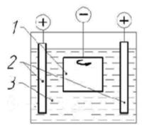
Fig. 6. Schemes of galvanic metallization with full immersion of the EI casting; 1 – EI Casting; 2 – electrodes; 3 – electrolyte bath
