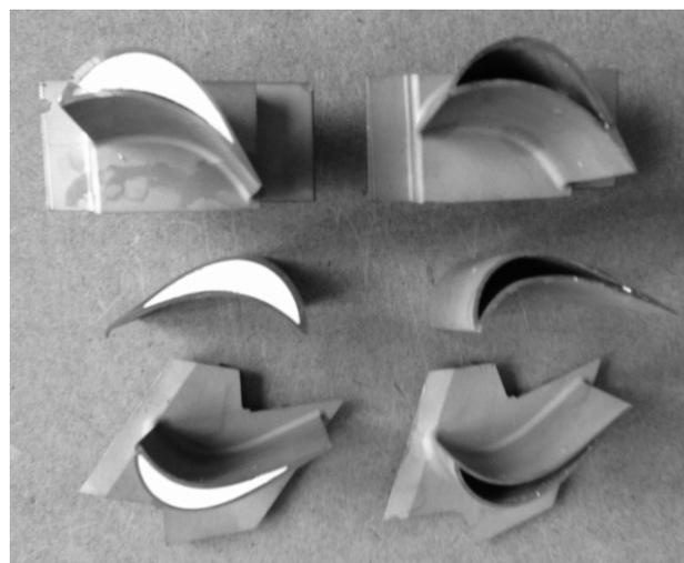
Fig. 4. Specimens before and after core removal
