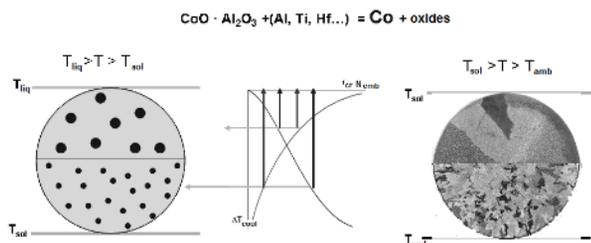
Fig. 11. Effect of supercooling on nucleation in casting of nickel based superalloys with refining coating
