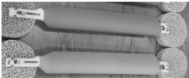
Fig 1. Cores after coating with 5 and 10 % mixture of  $\text{CoAl}_2\text{O}_4$
