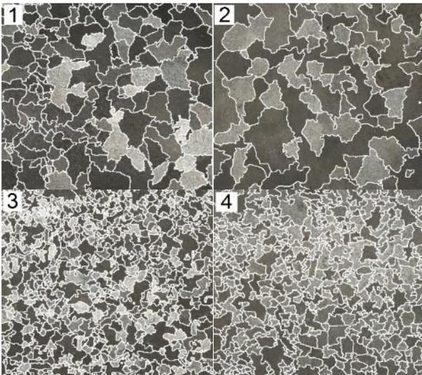
Fig. 6. Macrostructure comparison of specimens from sample 2: 1 – top inner (core), 2 – top outer (mould), 3 – bottom inner (core), 4 – bottom outer (mould)
