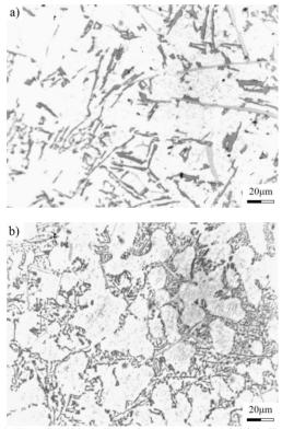
Fig. 6. EN AC-AlSi11 alloy microstructures: a) initial alloy, b) alloy after soft annealing treatment performed according to the variant 9
