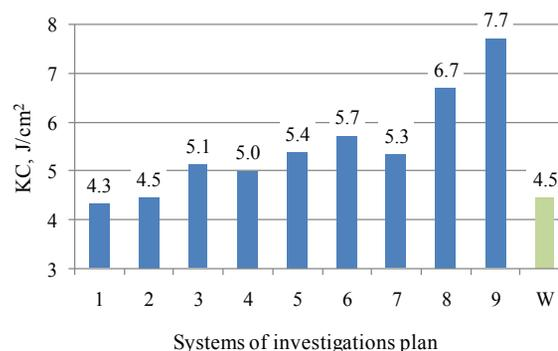
Fig. 2. Impact strength KC after the soft annealing treatment of the EN AC-ALSi11 alloy
