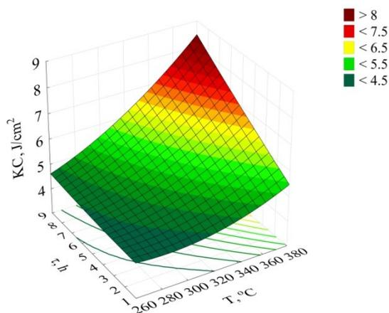
Fig. 3. The effect of soft annealing treatment temperature and time on the impact strength KC of the EN AC-ALSi11 alloy
