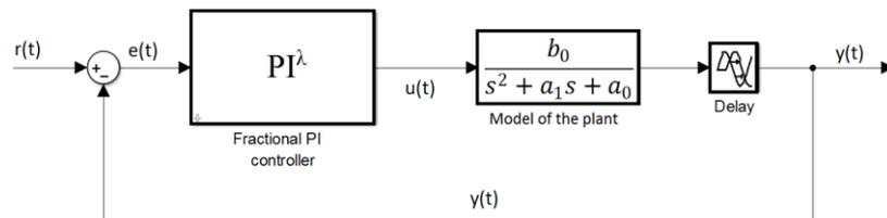
Fig. 1. Matlab-Simulink diagram of the considered control system
