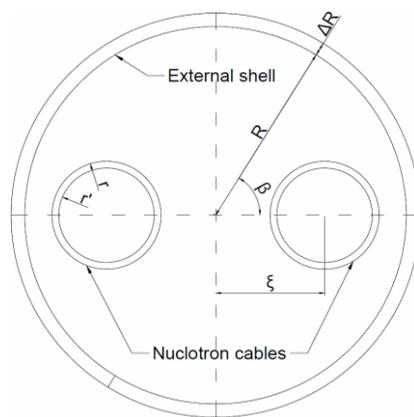
Fig. 1. Geometrical dimensions of the considered line
