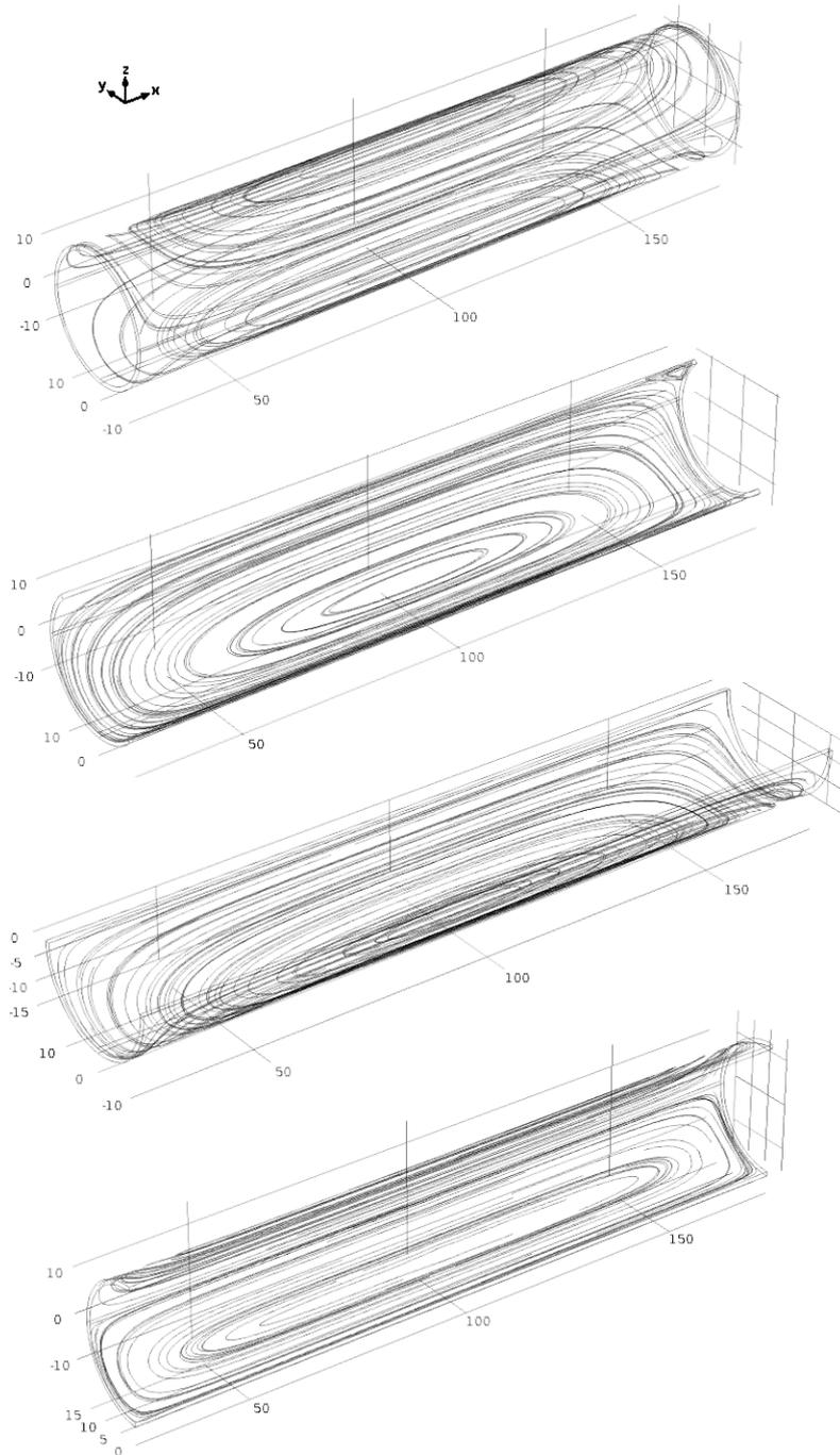
Fig. 5. Isometric view of streamlines of eddy currents for (top to bottom) full shell, split shell with angle  $\beta$  of 45°, 0°, 90°
