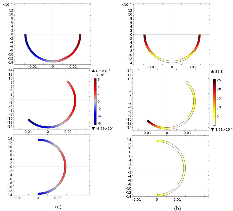
Fig. 4. Distribution of eddy currents density  $j$  in  $A/m^2$ : (a) and heat generation caused by them in  $W/m^3$ ; (b) shown on the cross-section of the split shell with angle  $\beta$  of (top to bottom)  $0^\circ$ ,  $45^\circ$ ,  $90^\circ$
