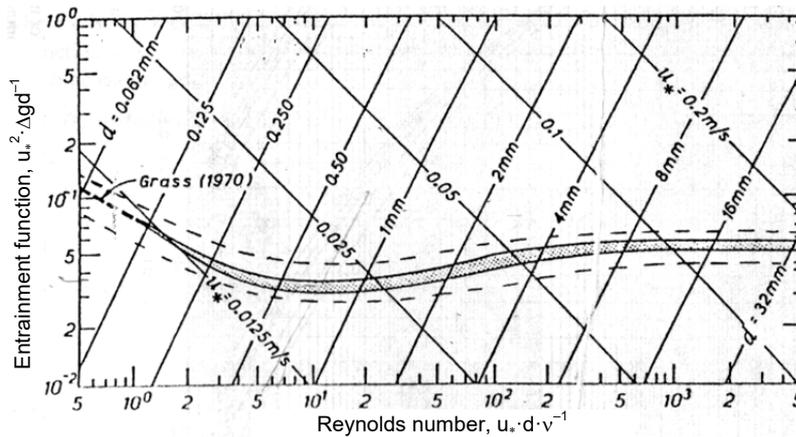
Fig. 1. Shields's curve:  $u_*$  = critical velocity,  $\rho_s$  = sediment density,  $d$  = diameter size of sediment,  $\nu$  = kinematics viscosity; source: BREUSERS, RAUDKIVI [1991]
