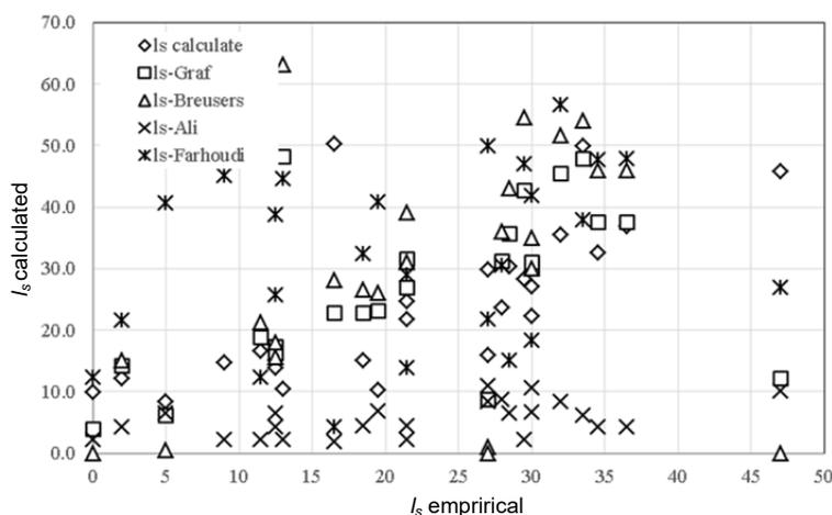
Fig. 13. Comparison between calculated depth of scour ( $d_s$ ) and experimental given by earlier researcher; source: own study
