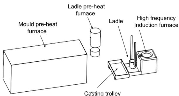
Fig. 1. Casting furnace and set-up for evaluating effects of variations originating from casting practice
