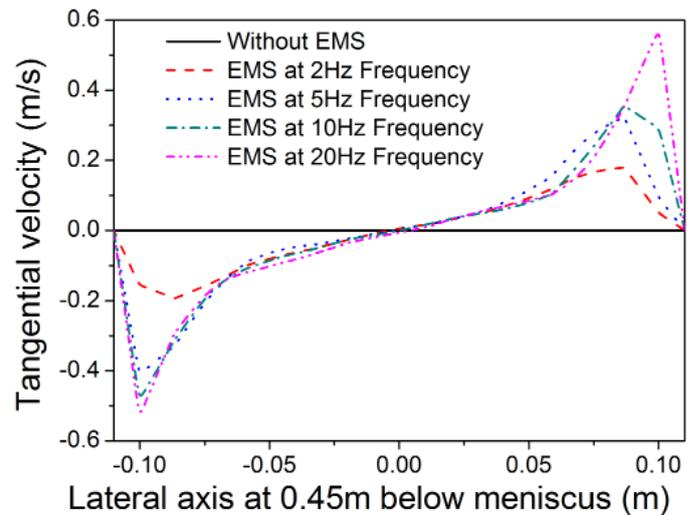
Fig. 10. Tangential velocity for different frequencies
