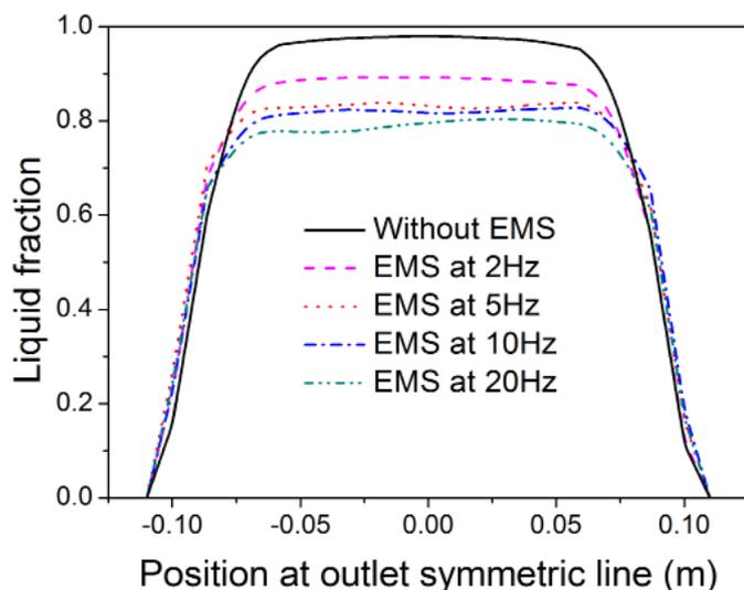
Fig. 8. Liquid fraction at mold outlet symmetric line
