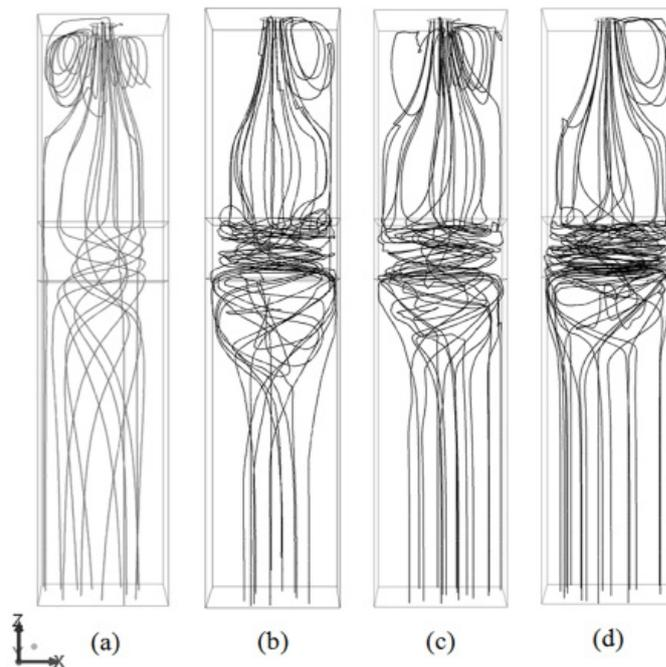
Fig. 12. Fluid flow pathlines during solidification with EMS at magnetic flux density (a) 0.05 T (b) 0.10 T (c) 0.15 T (d) 0.20 T
