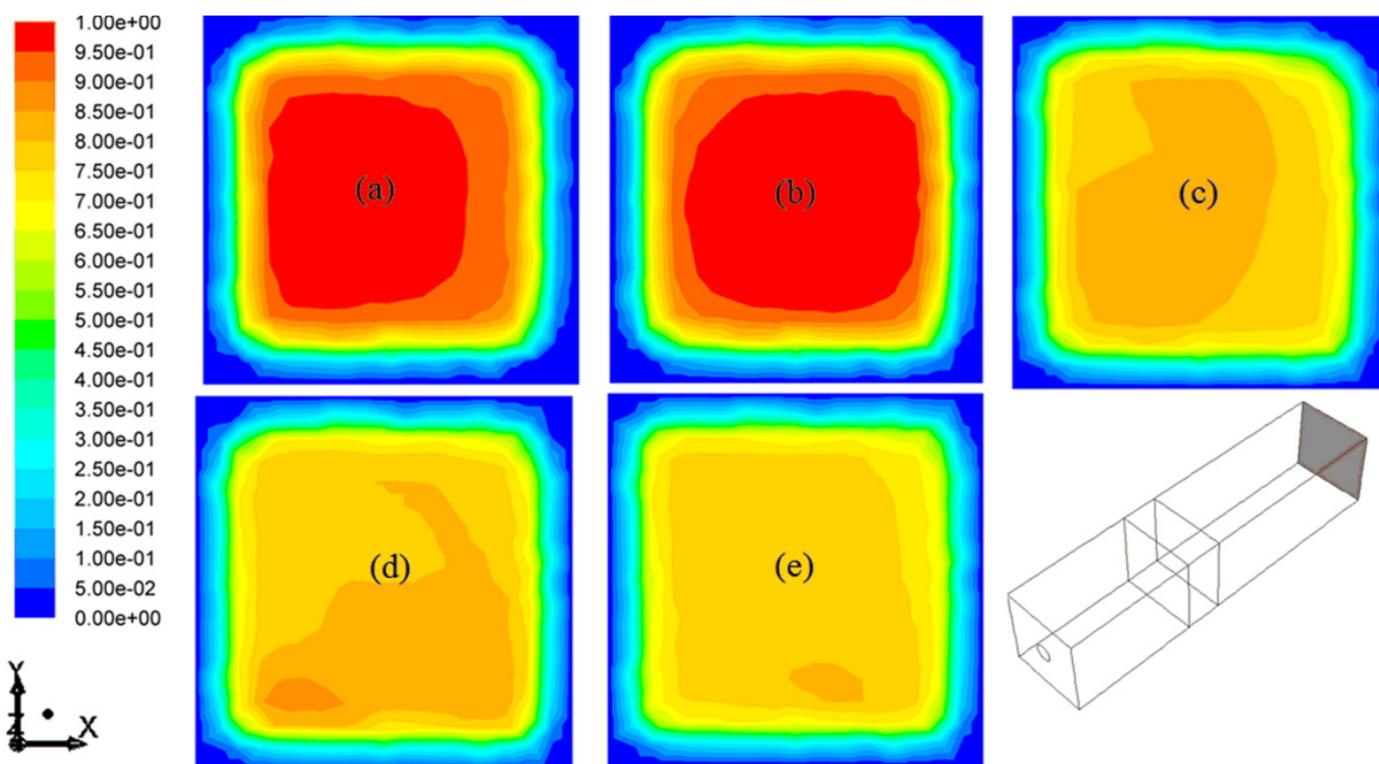
Fig. 13. Liquid fraction at mold outlet (a) Without EMS, and with EMS at magnetic flux density (b) 0.05 T (c) 0.10 T (d) 0.15 T (e) 0.20 T
