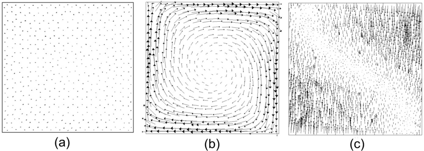
Fig. 3. Velocity vector for fluid flow (a) with solidification (b) with electromagnetic field, and (c) Vector distribution of Lorentz force under electromagnetic field
