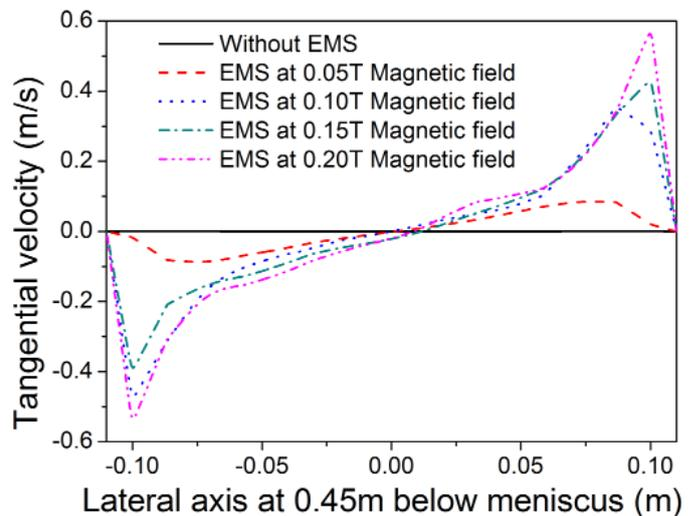
Fig. 16. Tangential velocity for different magnetic flux densities
