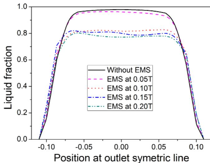
Fig. 14. Liquid fraction at mold outlet symmetric line
