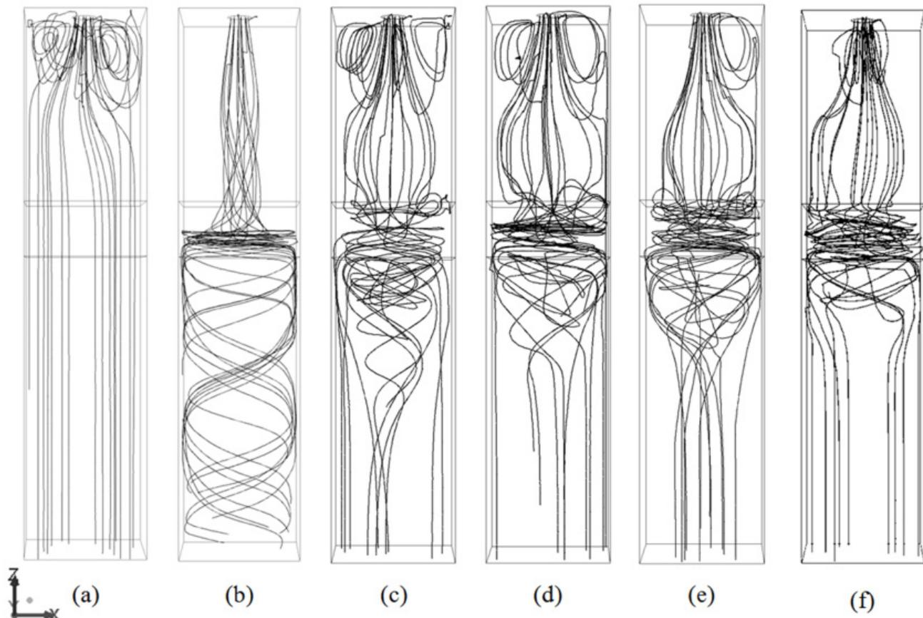
Fig. 6. Fluid flow pathlines (a) solidification without EMS (b) EMS without solidification, and solidification with EMS at frequency (c) 2 Hz (d) 5 Hz (e) 10 Hz (f) 20 Hz
