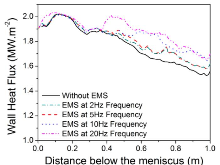
Fig. 11. Average wall heat flux for different frequencies
