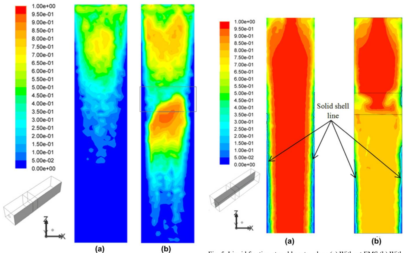
Fig. 4. Liquid fraction at mold wall (a) Without EMS (b) With EMS
