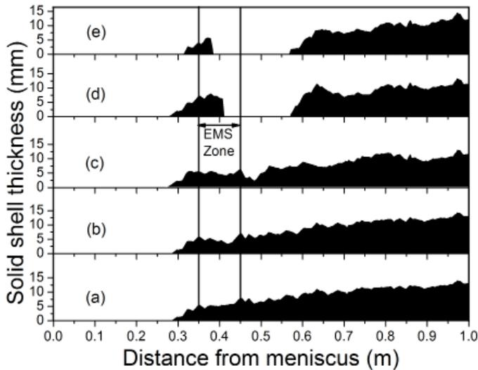
Fig. 9. Solid shell thickness at the center of mold wall, below the meniscus for cases (a) without EMS, and with EMS at frequencies (b) 2 Hz (c) 5 Hz (d) 10 Hz (e) 20 Hz
