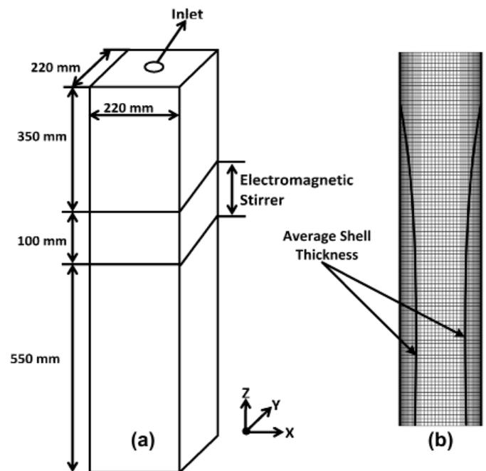
Fig. 1. (a) Model Geometry of billet caster mold (b) Computational grid at mold wall
