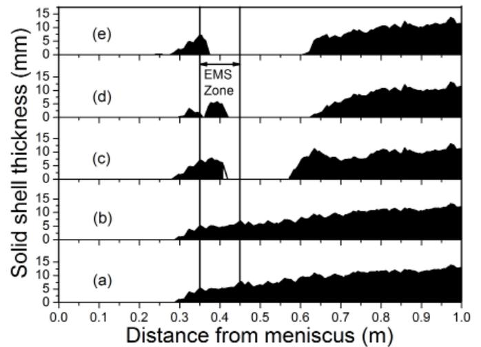
Fig. 15. Solid shell formation at the mold wall, below the meniscus for cases (a) Without EMS, and with EMS at magnetic flux density (b) 0.05T (c) 0.10T (d) 0.15T (e) 0.20T
