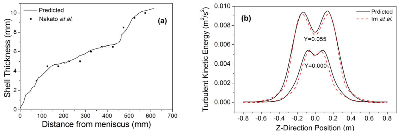
Fig. 2. Validation of (a) Solidification model (b) EMS model
