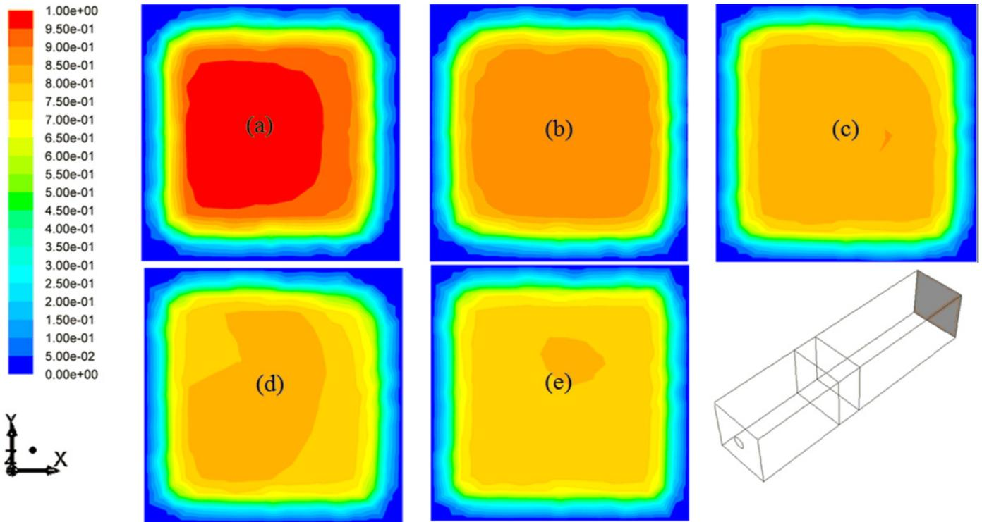
Fig. 7. Liquid fraction at mold outlet (a) without EMS, and with EMS at frequencies (b) 2 Hz (c) 5 Hz (d) 10 Hz (e) 20 Hz
