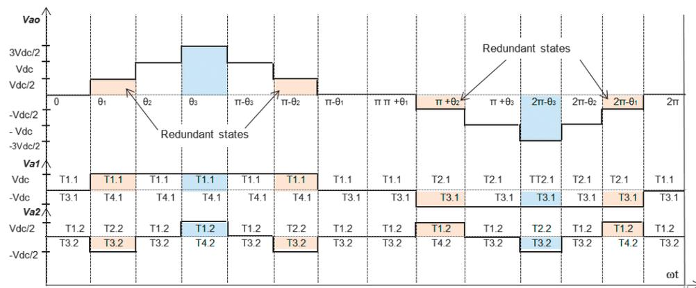
Fig. 3. Staircase CHB multilevel inverter output voltage
