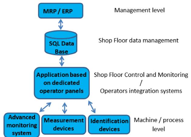
Fig. 4. Software configuration of the developed systems.
