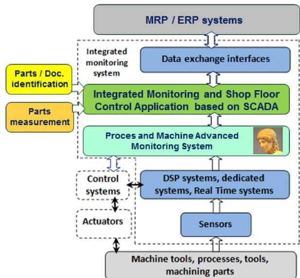
Fig. 2. Model of the integrated monitoring system developed in the research project.
