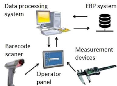
Fig. 6. The measurement system scheme.
