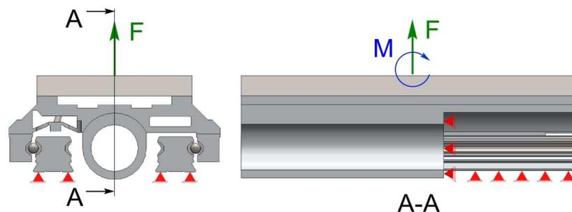
Fig. 7. Linear guide boundary conditions and loads
