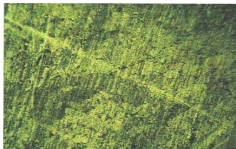
Fig. 2. Microstructure of weld No. 3, having highest pearlite content and CaF<sub>2</sub>
