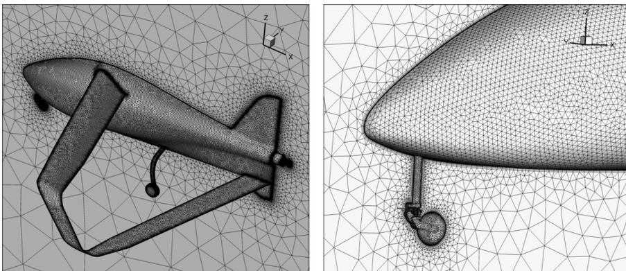
Fig. 5. An example of a computational mesh (IJWAC)
