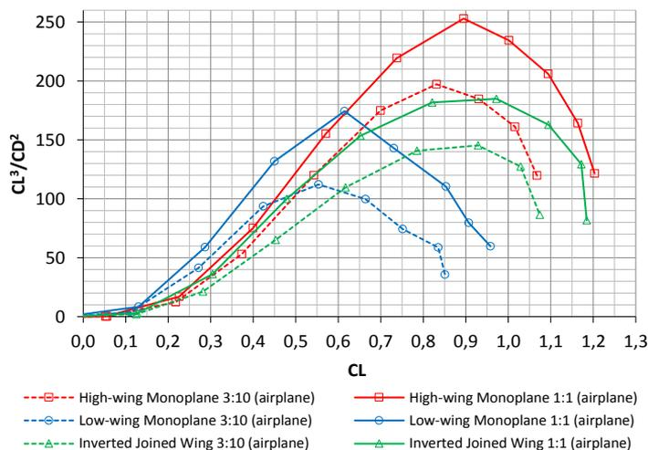
Fig. 11.  $CL^3/CD^2$  ratio vs.  $CL$  for all complete airplanes models
