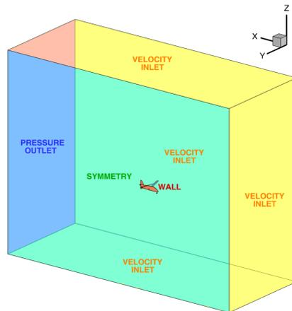
Fig. 4. An example of a computational domain with assumed boundary conditions
