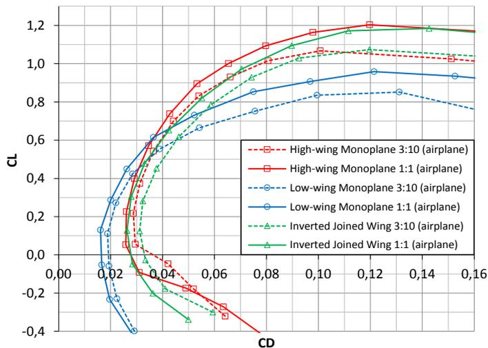
Fig. 13.  $CL(CD)$  curves (polars) for complete airplanes models
