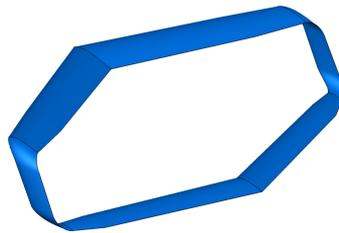
Fig. 2. Inverted joined wing isolated lifting surfaces model
