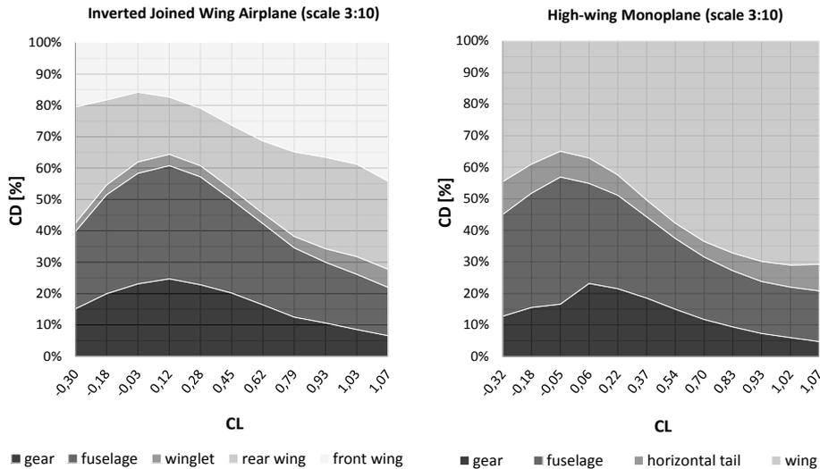
Fig. 14. The share of individual airframe parts in aerodynamic drag generation for inverted joined wing and ultralight high-wing monoplane – complete airplanes models (scale 3:10)
