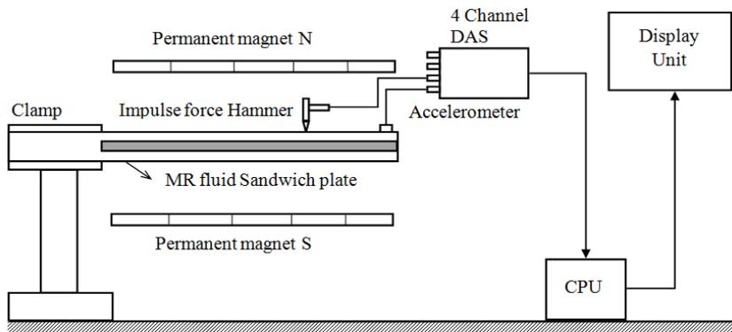
(b) Block diagram of the experimental setup of a clamped free (CFFF) fully treated laminated composite MR fluid sandwich plate
