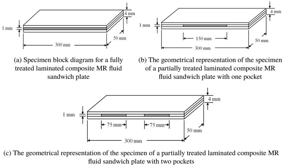
Fig. 1. The fully and partially treated laminated composite MR fluid sandwich plate
