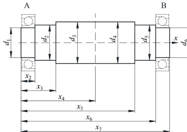
Fig. 4. Draft of a model shaft
