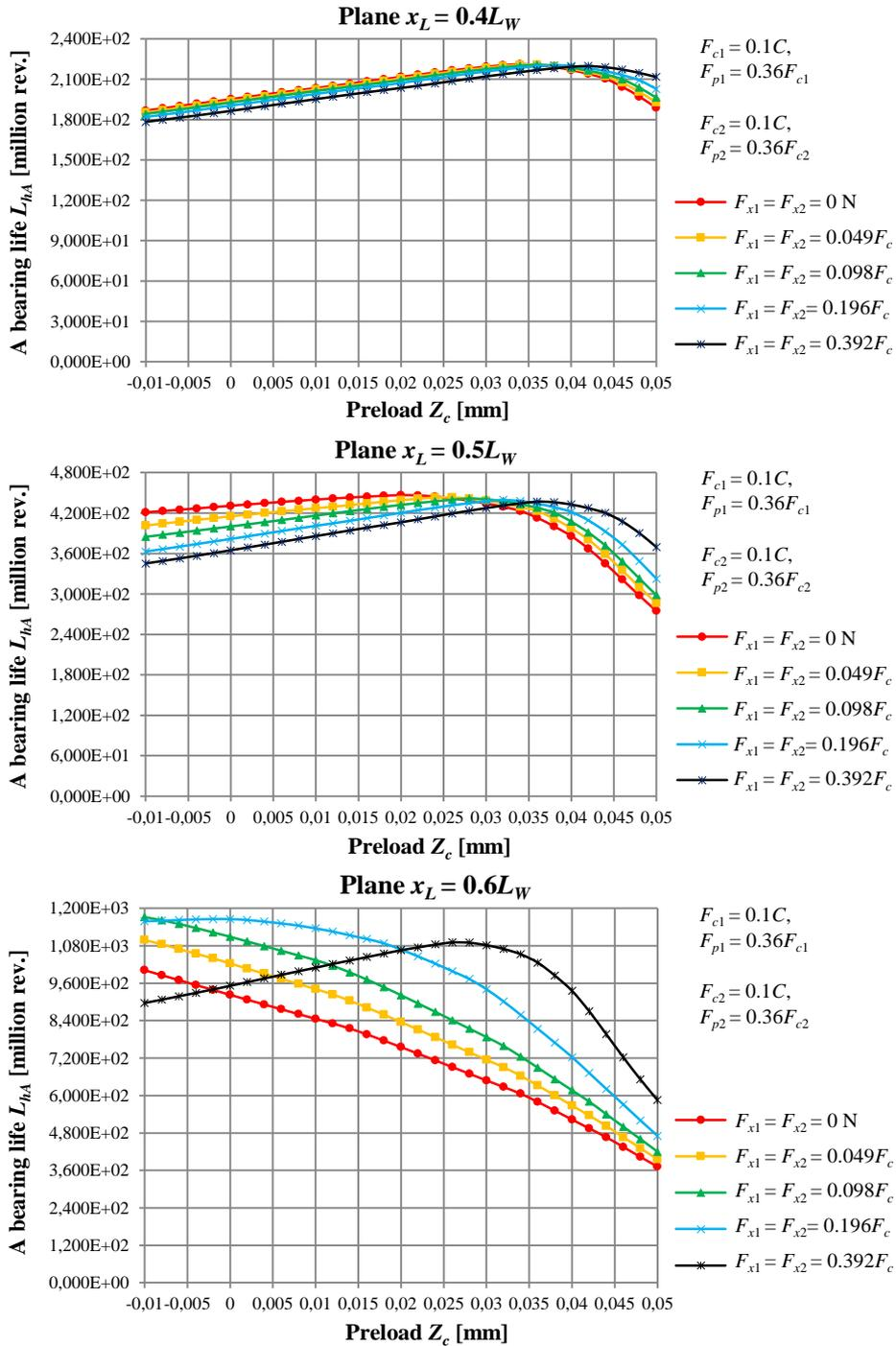
Fig. 6. Fatigue life of bearing A
