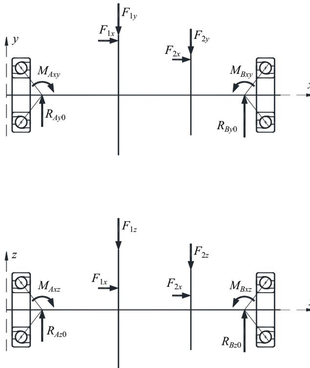
Fig. 2. Calculation scheme for transverse reactions of supports
