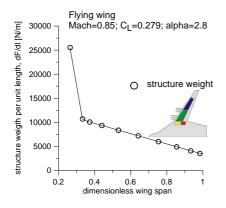
Fig. 13. Structure empty weight per unit length, from [4]
