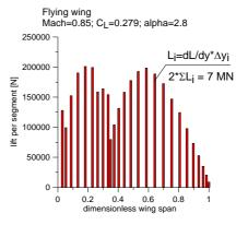
Fig. 12. Lift per segment, from [4]
