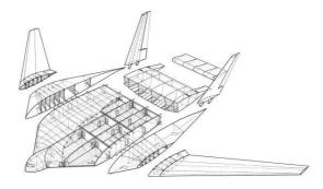
Fig. 5. 3D model of VELA3 - main structure segments [4]
