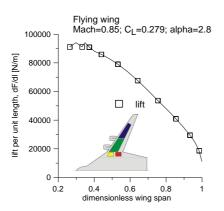
Fig. 11. Lift per unit length, from [4]
