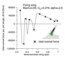
Fig. 16. Total normal force (Lift minus weight of structure+engine+fuel) per unit length, from [4]
