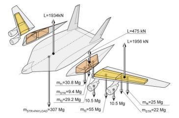
Fig. 20. Forces acting on wing (zero-order approximation), [4]
