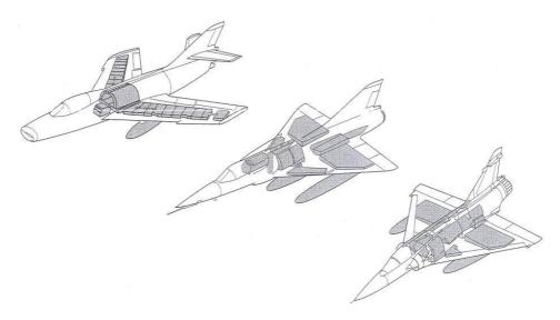
Fig. 1. Evolution of typical fuel tank layouts in military aircrafts [2]
