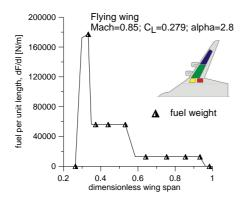
Fig. 15. Fuel weight per unit length, from [4]
