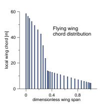
Fig. 9. Flying wing chord spanwise distribution, from [4]
