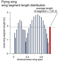
Fig. 10. Flying wing lateral segment length distribution, from [4]
