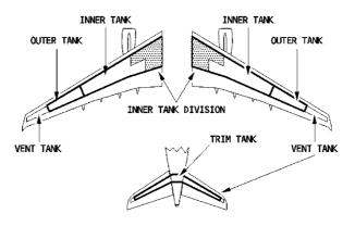
Fig. 2. Fuel tanks location of example airliner [3]
