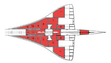
Fig. 3. Location of Concorde's fuel tanks [5]
