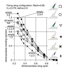
Fig. 18. Comparison of bending moments versus span (from [4])
