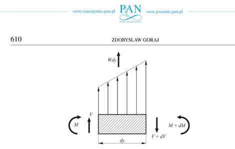
Fig. 7. Beam model of the wing spar showing bending moments and shear forces over an infinitesimal element
