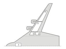
Fig. 6. Fuel tank arrangement. Wing tanks (1-4) and trim tanks (5) are shown
