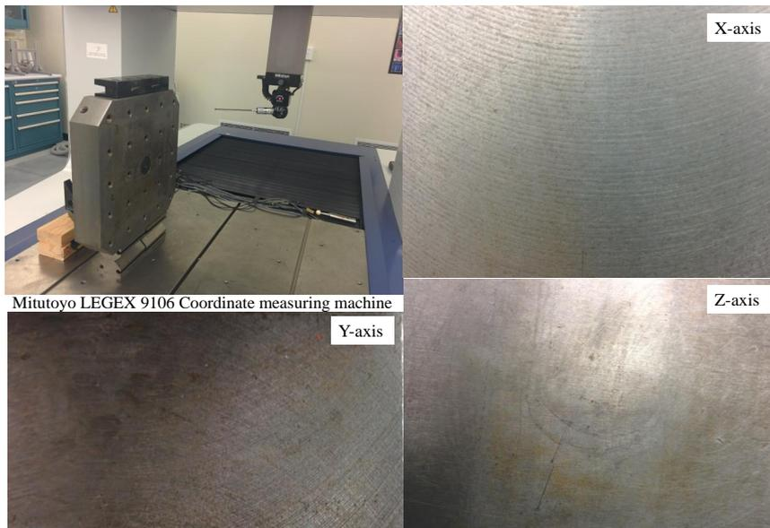
Fig. 8. The Coordinate Measuring Machine (CMM) and surface quality at X-, Y- and Z-direction
