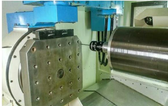
Fig. 1. Probing on a WCBXFZYT machine tool
