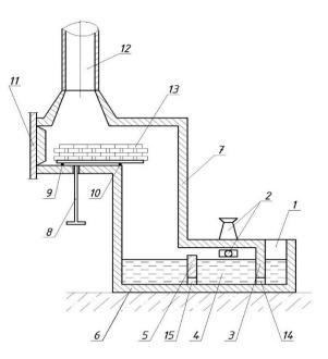
Fig. 1. Experimental gas-fired shaft-reverberatory furnace: 1 –
