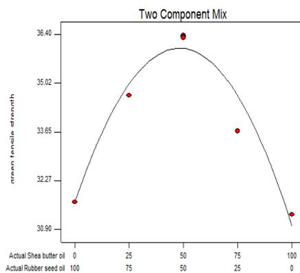
Fig. 31. 3% Oil in Sand: Green Tensile Strength
