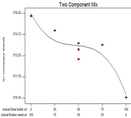
Fig. 20. 0.5% Oil in Sand: Dry Compressive Strength
