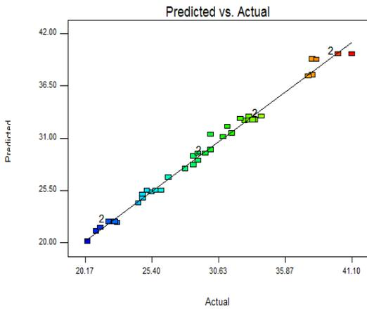
Fig. 8. Predicted vs Actual Response for Green Compressive Strength
