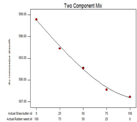
Fig. 23. 2% Oil in Sand: Dry Compressive strength
