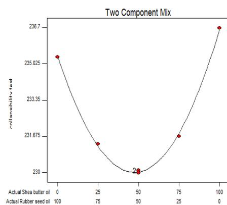
Fig. 47. 2.0% Oil in Sand: Collapsibility
