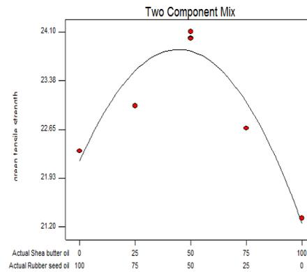
Fig. 27. 1% Oil in Sand: Green Tensile Strength
