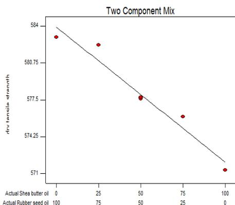
Fig. 36. 2.5% Oil in Sand: Dry Tensile Strength
