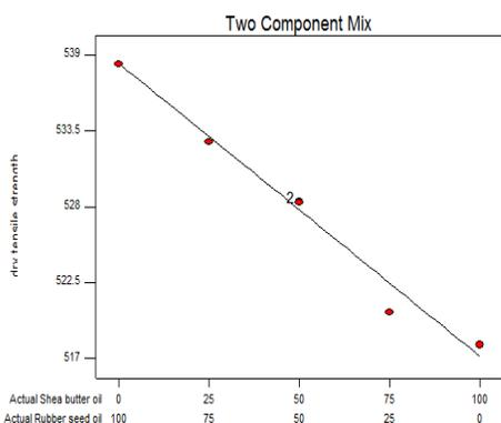
Fig. 32. 0.5% Oil in Sand: Dry Tensile Strength
