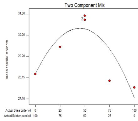
Fig. 29. 2.0% Oil in Sand: Green Tensile Strength
