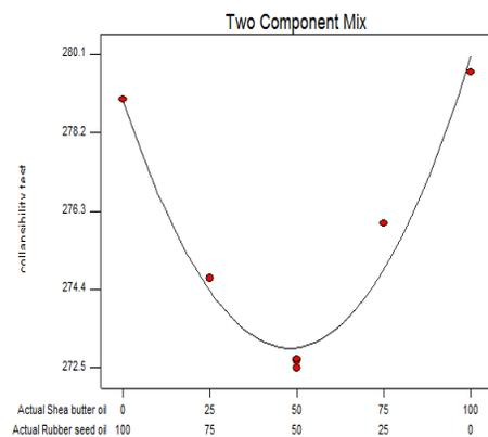
Fig. 45. 1% Oil in Sand: Collapsibility
