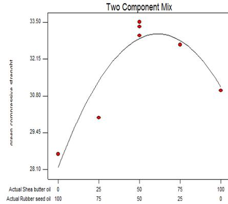
Fig. 17. 2% Oil in Sand: Green Compressive Strength
