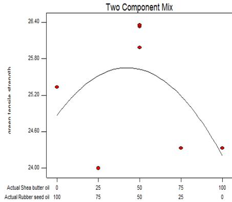
Fig. 28. 1.5% Oil in Sand: Green Tensile Strength
