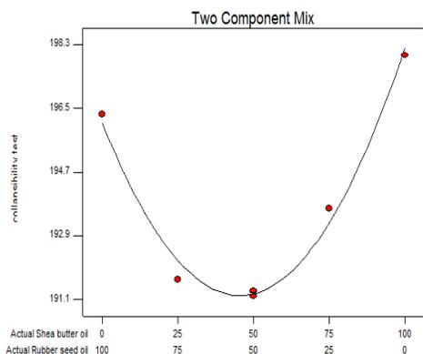
Fig. 48. 2.5% Oil in Sand: Collapsibility
