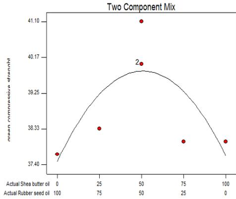
Fig. 19. 3.0% Oil in Sand: Green Compressive Strength
