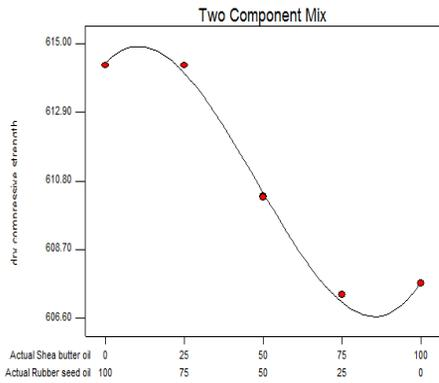
Fig. 24. 2.5% Oil in Sand: Dry Compressive Strength
