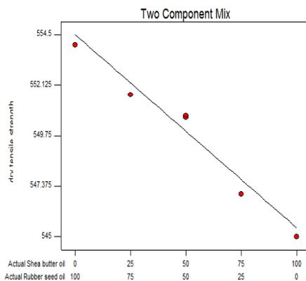
Fig. 33. 1% Oil in Sand: Dry Tensile Strength
