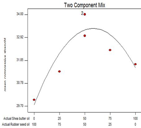
Fig. 18. 2.5% Oil in Sand: Green Compressive Strength
