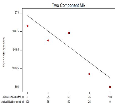
Fig. 34. 1.5% Oil in Sand: Dry Tensile Strength
