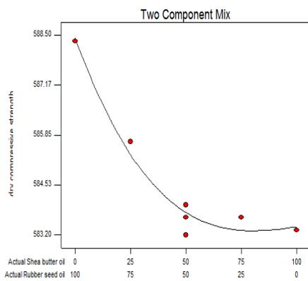
Fig. 22. 1.5% Oil in Sand: Dry Compressive Strength
