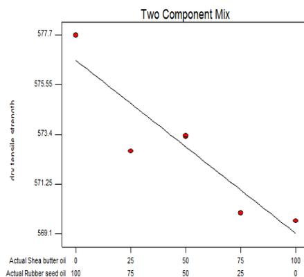
Fig. 35. 2% Oil in Sand: Dry Tensile Strength
