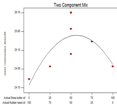
Fig. 15. 1% Oil in Sand: Green Compressive Strength
