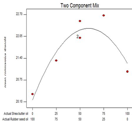
Fig. 14. 0.5% Oil in Sand: Green Compressive Strength
