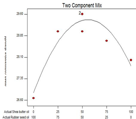
Fig. 16. 1.5% Oil in Sand: Green Compressive Strength
