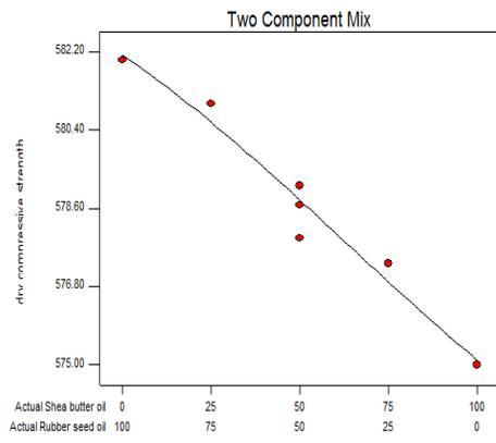
Fig. 21. 1% Oil in Sand: Dry Compressive Strength
