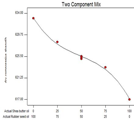
Fig. 25. 3% Oil in Sand: Dry Compressive Strength
