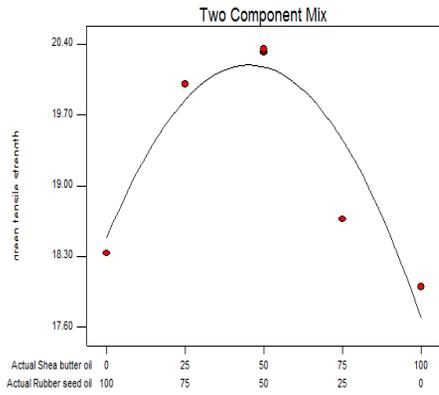
Fig. 26. 0.5% Oil in Sand: Green Tensile Strength
