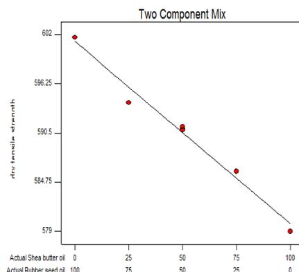
Fig. 37. 3% Oil in Sand: Dry Tensile Strength
