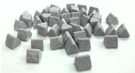
Fig. 2. Ceramic media CB 20T - density 2.4–2.7 kg/dm<sup>3</sup>
