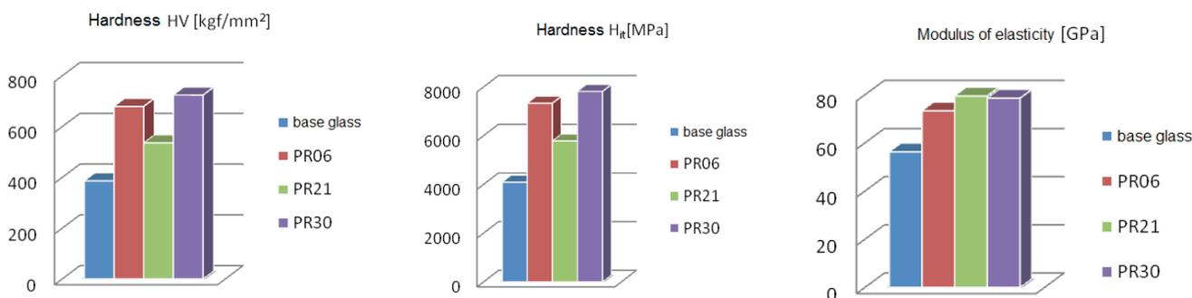
Fig. 2 The mechanical properties of the base glass samples and ZrO<sub>2</sub> coated samples: hardness HV, modulus of elasticity
