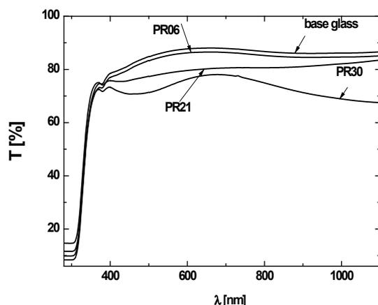
Fig. 3. Transmittance of glass samples coated with  $ZrO_2$
