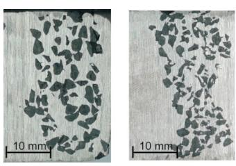
Fig. 3. Casting with locally reinforcement produced layer
