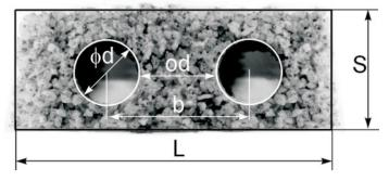
Fig. 1. Ceramic insert to form the composite layer
