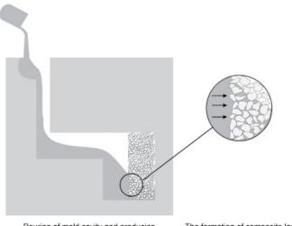
Pouring of mold cavity and producing a composite zone in casting
