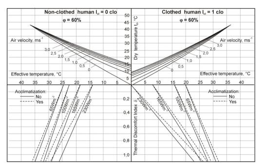
Fig. 3. The nomogram for thermal discomfort assessment, relative humidity  $\varphi = 60\%$
