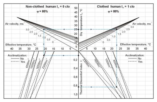
Fig. 4. The nomogram for thermal discomfort assessment, relative humidity  $\varphi = 80\%$
