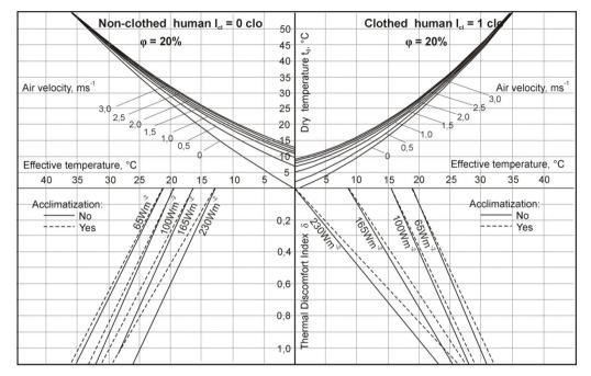
Fig. 1. The nomogram for thermal discomfort assessment, relative humidity  $\varphi = 20\%$
