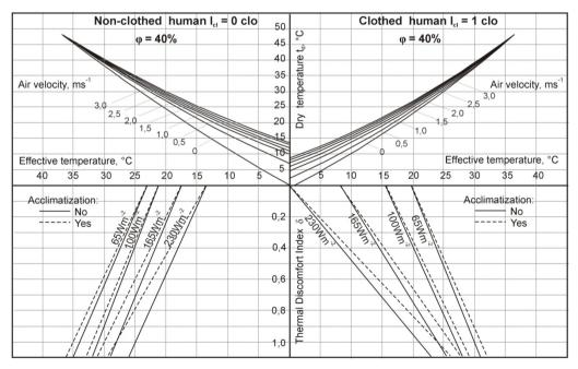
Fig. 2. The nomogram for thermal discomfort assessment, relative humidity  $\varphi = 40\%$
