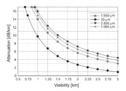
Fig. 10. Radiation attenuation versus visibility [38].
