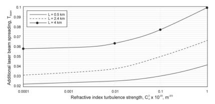
Fig. 7. Laser beam spreading vs. refractive index structure parameter for different propagation lengths and a beam wavelength of 1550 nm [28].
