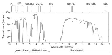
Fig. 4. Transmittance through the atmosphere as a function of wavelength.
