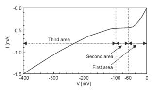
Fig. 17. A reverse dark current-voltage plot measured at 200 K. The background radiation was suppressed by 200 K cold shield. A physical photodiode area is  $0.03 \times 0.03$ mm<sup>2</sup>.
