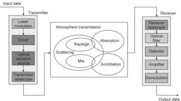
Fig. 2. Construction of an FSO data link [1].
