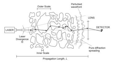
Fig. 6. Propagation of a laser beam through the turbulent atmosphere [28].
