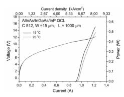
Fig. 14. Light-current and current-voltage characteristics of the Al0.48In0.52As/In0.53Ga0.47As/InP  $(\lambda = 9.2 \ \mu m)$  laser driven by 200 ns pulses with a repetition rate of 1 kHz [45].
