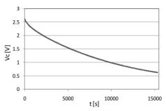
Fig. 5. A discharging curve of the tested supercapacitor, DRL 2.7V 10F type, through the loading resistance of 1 k $\Omega$ .
