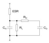
Fig. 3. A two-branch model of supercapacitor.
