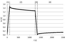
Fig. 2. A change of voltage between supercapacitor terminals during charging (1), when disconnected (2), (4) and during discharging (3).
