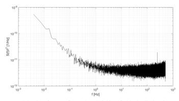
Fig. 7. Power spectral density of current fluctuations S(f) identified in the discharging current I of a DRL 2.7V 10F specimen when discharged through the loading resistance 1 k $\Omega$ . Power spectrum estimated in each time interval was normalized by the square of the discharging current.
