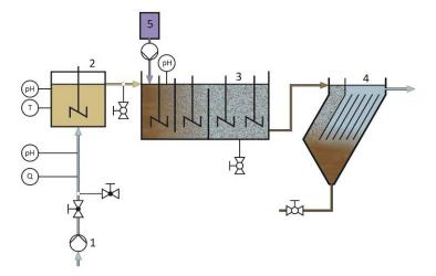
Fig. 1. Schematic of the test flow system with supply pump (1), raw water tank (2), flocculation chamber (3), settling tank (4), system for dosing coagulant into the rapid mixing chamber (5) and flow (Q), pH, and temperature (T) measurement points
