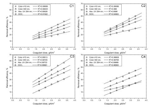
Fig. 2. Effect of coagulant dosage on coagulation effectiveness with C1-C4 coagulants for the batch mode system
