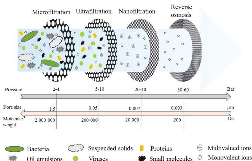
Fig. 1. Comparison of pressure filtration methods (own analysis)
