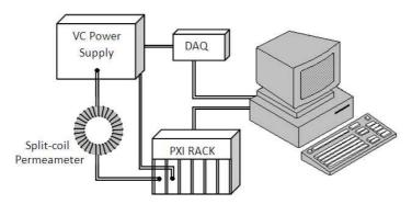
Fig. 6. The split-coil permeameter measurement setup.
