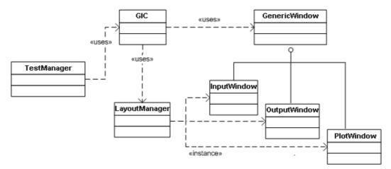
Fig. 5. Abstract Factory Pattern for the GUI engine.
