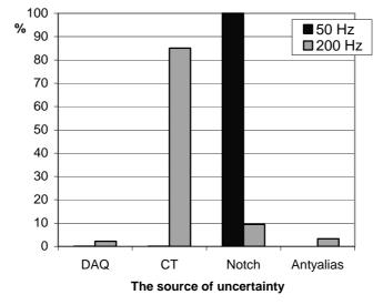
Fig. 7. Share of main uncertainty components in the complex uncertainty for two frequencies: 50 and 200 Hz DAQ - data acquisition card, CT - current transducer, Notch - notch filter, Antyalias - antyalising filter.
