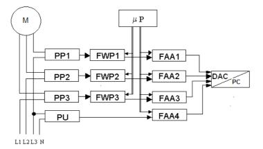
Fig. 2. Current measurement system for induction motor (where: M – induction motor; μP – microprocessor; PP1– PP3 – transducers for current measurements; PU – transducer for voltage measurements; FAA1-FAA4 – antialiasing filters; FWP1-FWP4 – narrow band filters; A/D – data acquisition card; PC – computer).
