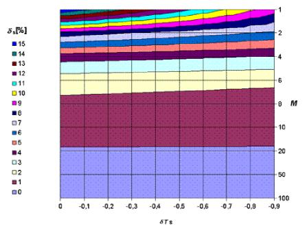
Fig. 7. Chart of charge relative error  $\delta_s$  on ADC sampling offset  $\delta T_s$  and rate *M*.
