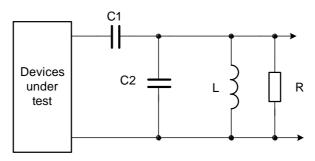
Fig. 1. Standard input circuit of discharge meter.
