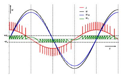
Fig. 2. Time plot of driving and void voltage, current trough the dielectric mass.
