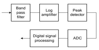
Fig. 4. Improved partial discharge meter with logarithmic amplifier peak detector and ADC.
