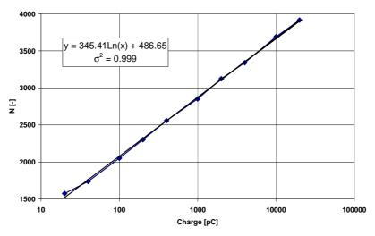
Fig. 8. Partial discharge meter transfer characteristic.
