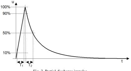
Fig. 3. Partial discharge impulse.
