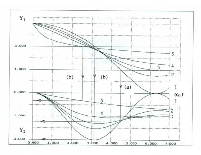
Fig. 1. The curves  $Y_1(t \cdot \omega_0)$  and  $Y_2(t \cdot \omega_0)$  for transfer function (15) and five values of B = 0,0.2,0.35.0.65,3. The bigger B the bigger the digit indicating the respective curve.
