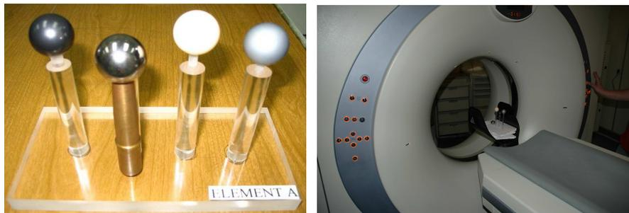
Fig. 1. Reference balls and their test using computer tomography.
