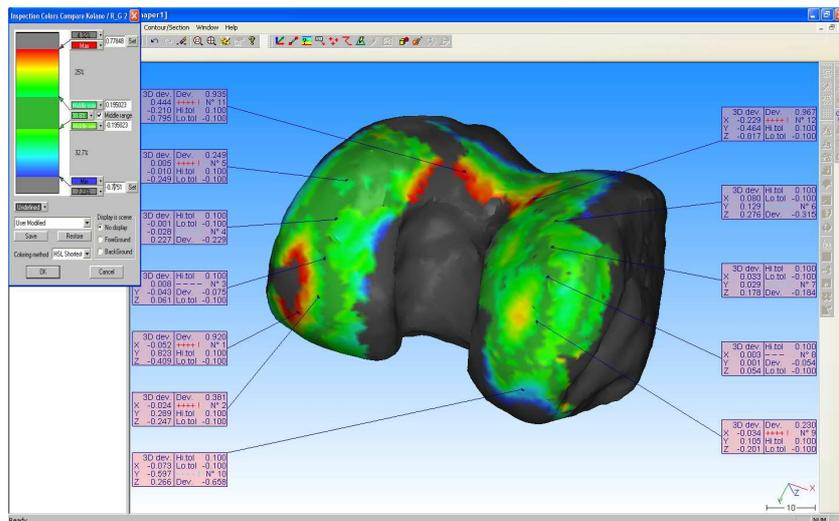
Fig. 15. Knee-joint – the map of deviations of shape mapping as the comparison of the imposition of the surface derived from the CT studies with the surface obtained from studies on CMM.
