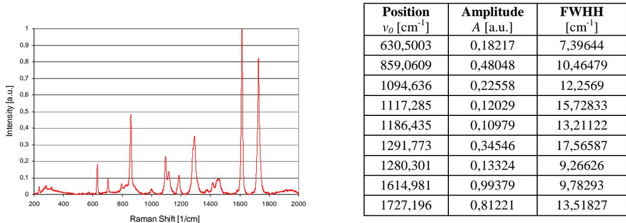
Fig. 9. The main parameters (right) of the exemplary Raman spectrum (left) estimated by the described algorithm.
