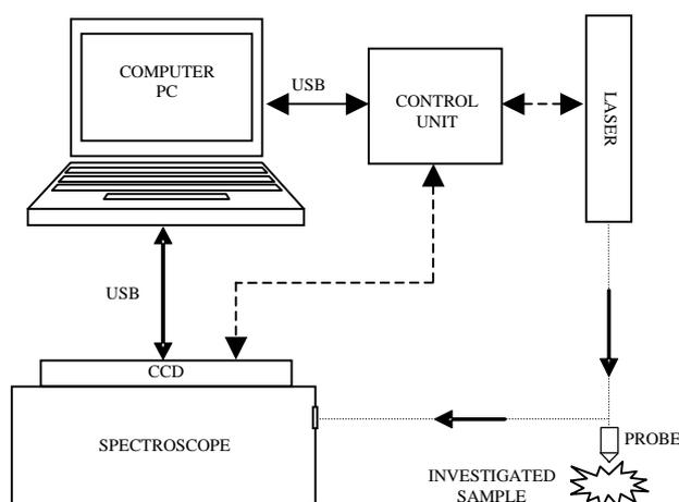
Fig. 2. Block diagram of a portable Raman spectrometer.
