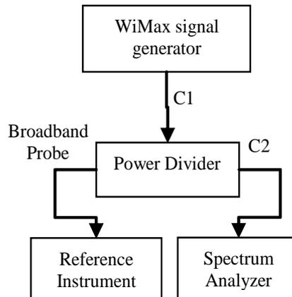
Fig. 2. Measurement setup for the characterization of the WiMAX radiated emissions.
