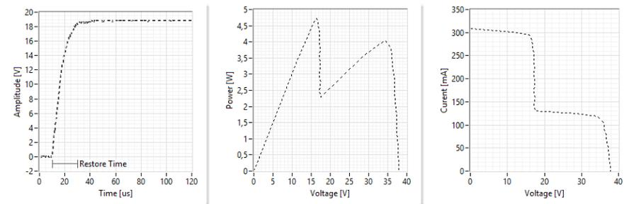
Fig. 9. The response to a short load pulse: voltage (left), power (middle), current – according to the measured I–V curve for partial shading conditions (right).
