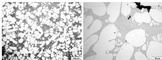
Fig. 14, 15. Structure inoculated by 0,05 % AlTi5B1
