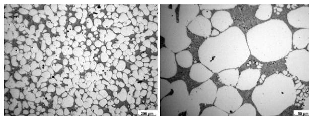
Fig. 20, 21. Structure inoculated by 0,2 % AlTi5B1
