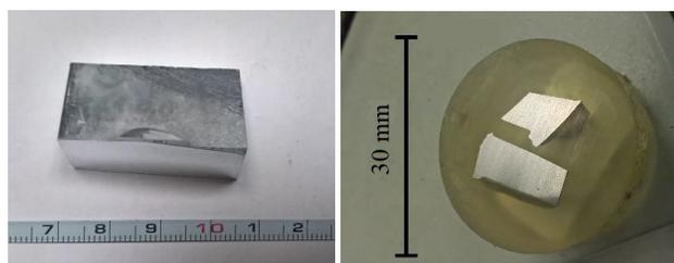
Fig. 10, 11. Preparation of samples for light microscopy
