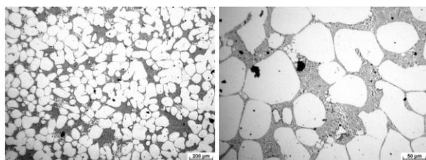
Fig. 12, 13. As cast structure without inoculation
