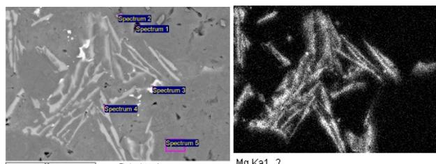
Fig. 6, 7. Studied structure (left) and mapping for magnesium (right)
