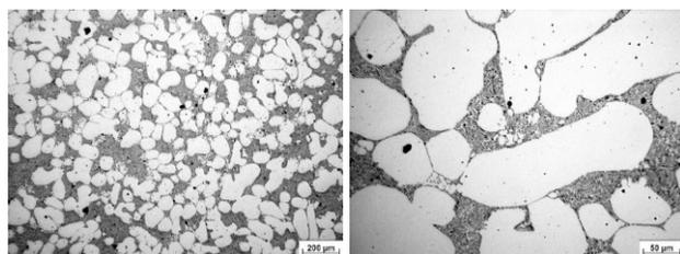
Fig. 16, 17. Structure inoculated by 0,1 % AlTi5B1
