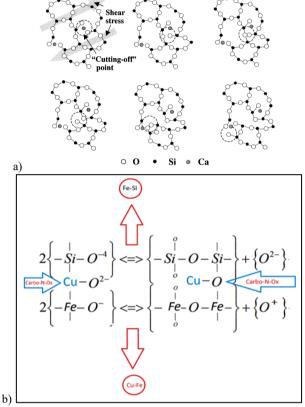
Fig 2. a) Mechanism of breaking silicon-oxygen anions according to Tanaka [5], b) Proposed reaction scheme for slag suspensionreagents of Carbo-N-Ox system [4]
