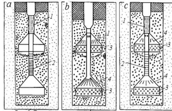
**Fig. 3. Bell type Water Well Construction:**
