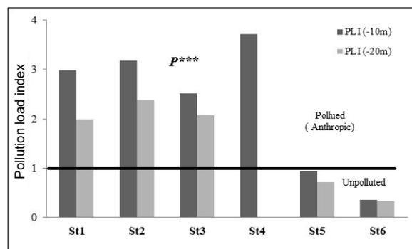
Fig. 4. Variations of the pollution load index (*PLI*) in the sediment samples collected from various stations; St1–St6 as in Fig. 2; source: own study
