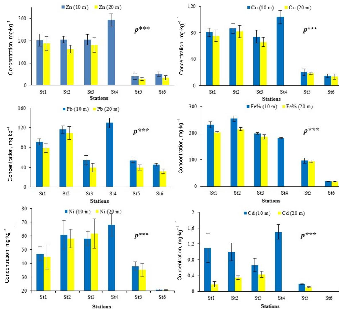
Fig. 2. Average concentrations of metals in sediments (mg·kg<sup>-1</sup> dry weight) of the six selected stations: Sidi Salem Beach (St1); Wadi Seybouse Beach (St2); Joinoville Beach (the industrial zone of Asmidal) (St3); harbour station (St4); Rizi Amor Beach (St5); Ain-Achir Beach (St6);  $p \leq 0.001$ ; source: own study
