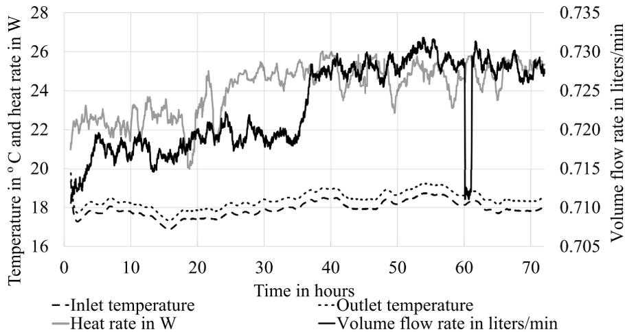
Figure 7: Measured temperatures and volume flow rate of the water in cooling cap together with heat rate – patient N1 .
