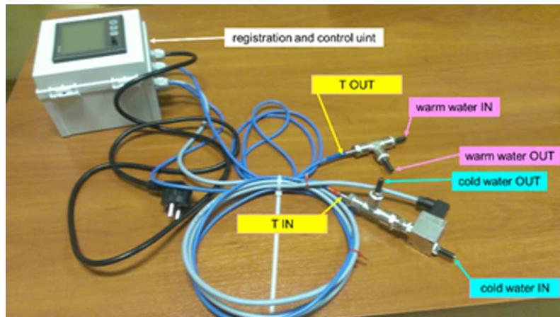
Figure 5: The water flow meter equipped with temperature sensors to monitor fluctuations of heat flux in the brain cooling process remotely.
