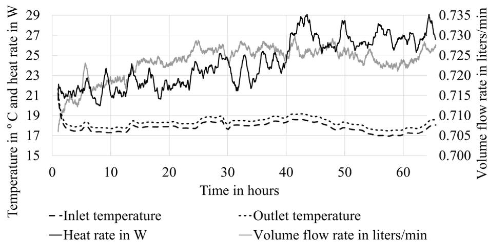
Figure 11: Measured temperatures and volume flow rate of the water in cooling cap together with heat rate – patient N3.
