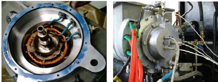
Fig. 2. Prototype and stator end of the HSPMG
