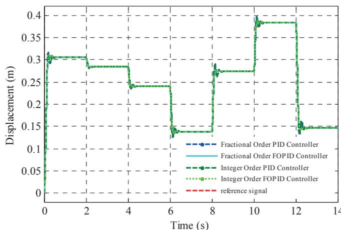
Fig. 8. System responses to multi-pulses position profile
