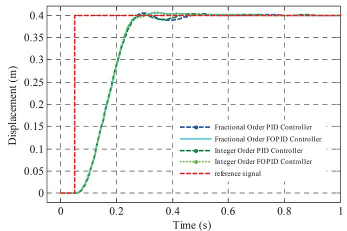
Fig. 7. System responses to step position profile
