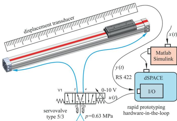
Fig. 2. Schematic diagram of pneumatic servo-drive
