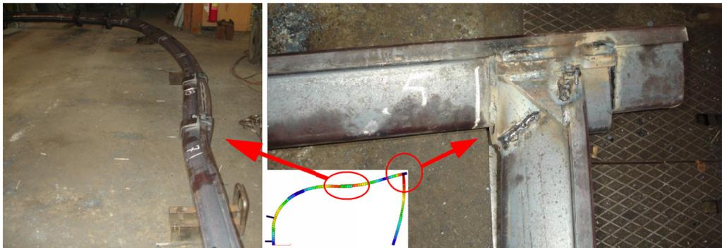
Fig. 9. Arch-rectangular support after tests and comparison with results of numerical modeling. Deformation of the canopy (on the left) and deformation of the canopy and prop connection (right)
