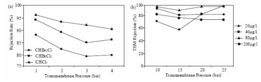
Fig. 3. Influence of transmembrane pressure, concentration and THM type on retention coefficient of THMs, (a) NF200 membrane and (b) DS5 membrane
