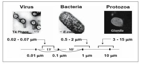
Fig. 1. Comparison of micro-organisms sizes with MF and UF membrane pore size
