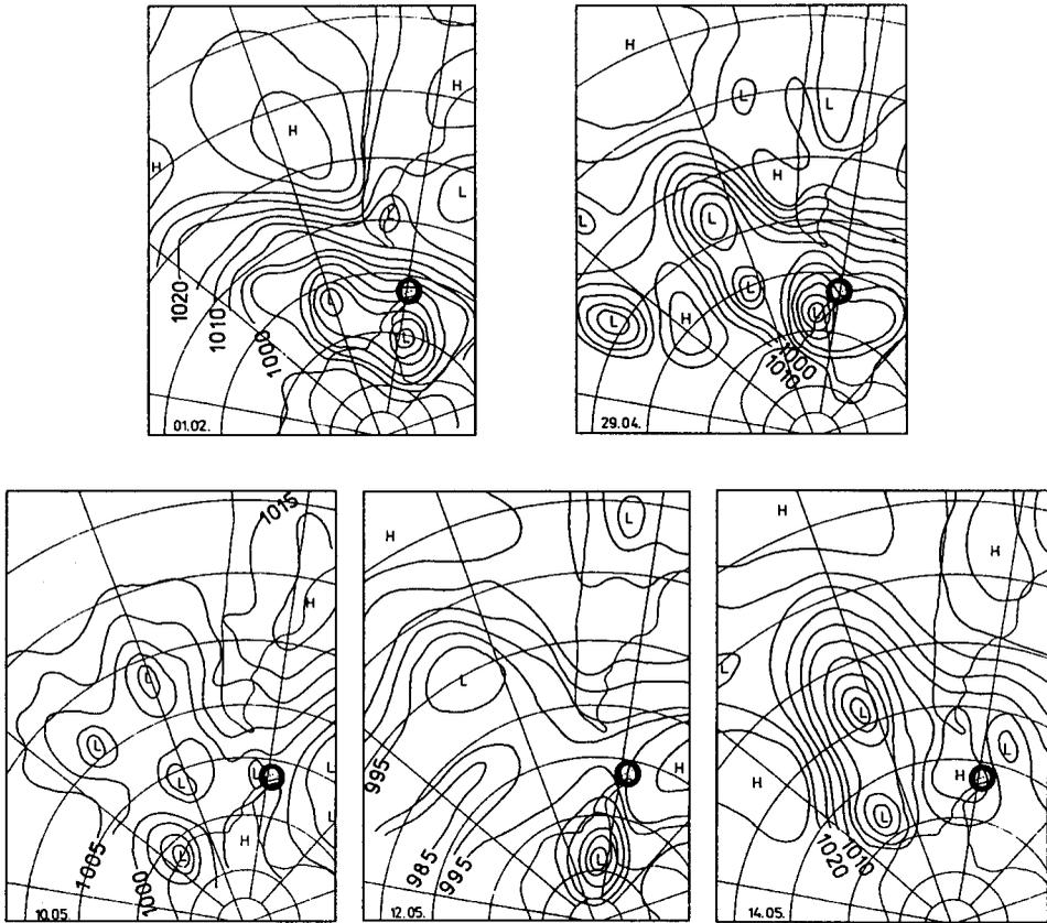
Fig. 2. Maps of air pressure distribution in the South Atlantic on days with selected weather conditions at the *Arctowski* Station in autumn 1991, according to the Chilean Navy Meteorological Survey; isobars in hPa.
