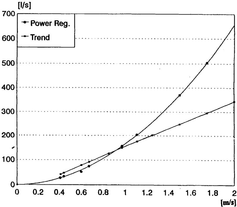
Fig. 7. Relation of water discharge and flow velocity, plotted as linear (trend) and power regression lines at Skamieniały Las Creek, site Limmigraf.
