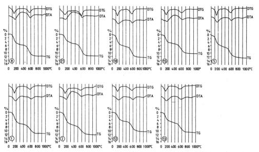
Fig. 3. Derivatograms of the glacial deposits of Petuniabukta. The fraction smaller than 0.002 mm. DTG: 1/5, DTA: 1/10, TG: 200 mg
