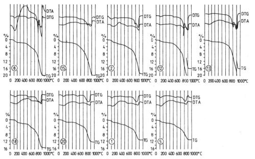
Fig. 2. Derivatograms of the glacial deposits of Petuniabukta. Natural samples. DTG: 1/5, DTA: 1/10, TG: 200 mg
