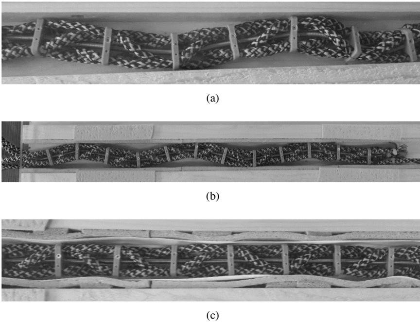
Fig. 6. Sample tracks for the robot to traverse: a) track made of wooden planks; b) track made of wooden planks, walls lined with sponges; c) track made of wooden planks, walls lined with sponges and Teflon tape
