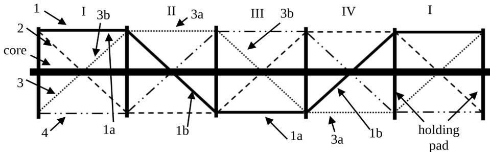
Fig. 1. Diagram of muscle attachment in the snake-like robot 1, 2, 3, 4 – subsequent cables with McKibben muscles; 1a – working part of cable 1 (McKibben muscle), 1b – non-working part of the cable 1, 3a – working part of cable 3 (McKibben muscle), 3b – non-working part of the cable 3
