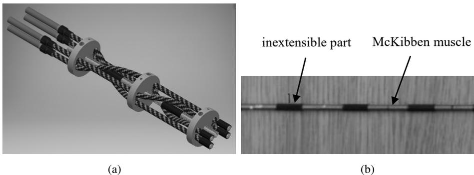
Fig. 2. a) sample structure of a snake-like robot based on McKibben muscles; b) cable with McKibben muscles used to construct the robot
