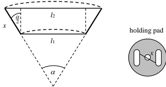
Fig. 3. Simplified model of a single section of the robot
