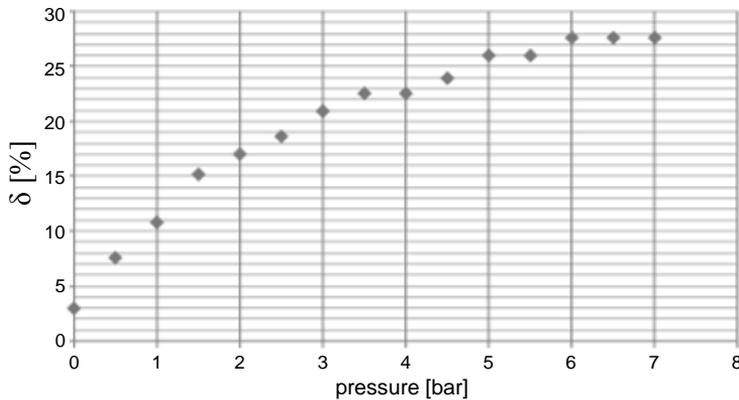
Fig. 4. Muscle shortening in the function of pneumatic pressure
