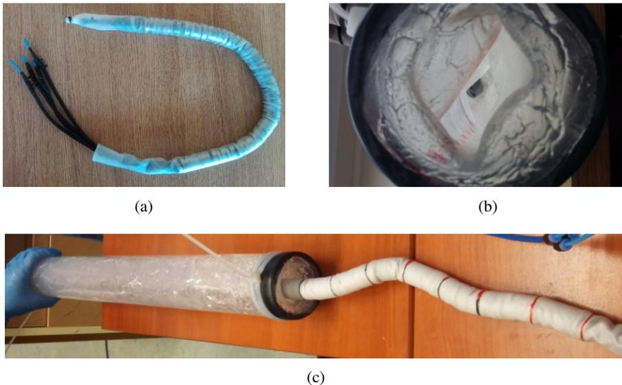
Fig. 9. a) Generation II snake-like robot with a pneumatic drive; b) front view of the tunnel simulating an environment with high damping and elasticity coefficients; c) robot introduced into the tunnel
