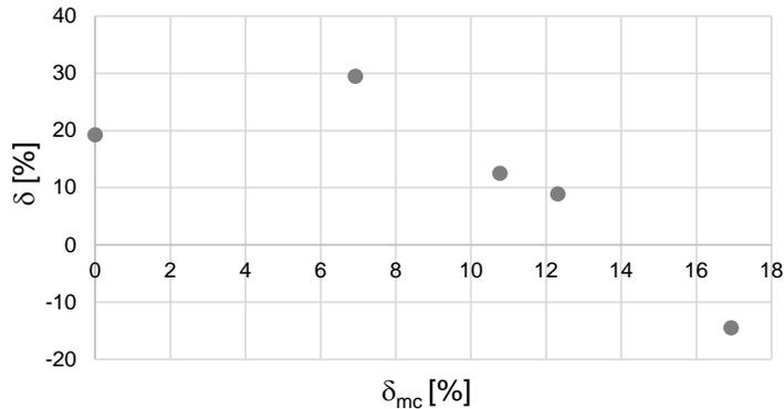
Fig. 5. Plot of the function of muscle shortening depending on the tension of the McKibben muscle core ( $\delta_{mc}$ )
