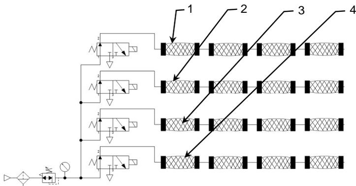
Fig. 7. The pneumatic schema of the snake-like robot
