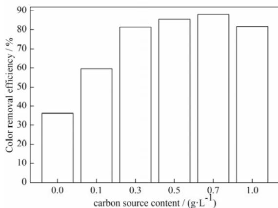
Fig. 4. Color removal rate with different carbon source content of influent in BES
