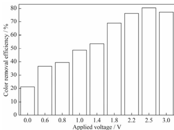
**Fig. 2.** Color removal efficiency at different applied voltages in BES
